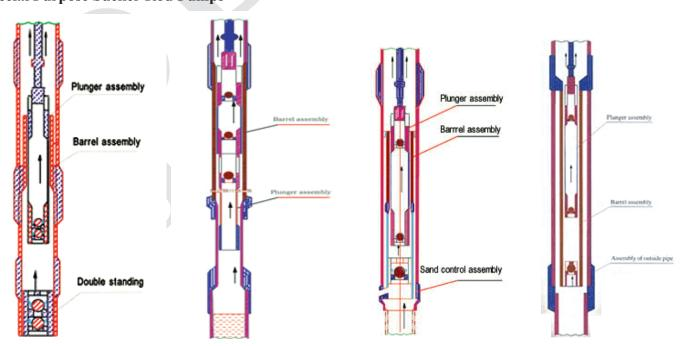
There are some special purpose subsurface pumps of other structure. Special purpose subsurface pumps of different sizes and usages according to customers' requirements can be designed and manufacture.
